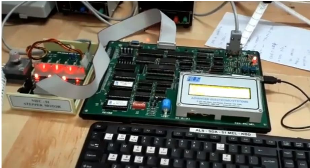
Figure 8 : Based on the activation of windings stepper motor rotating
