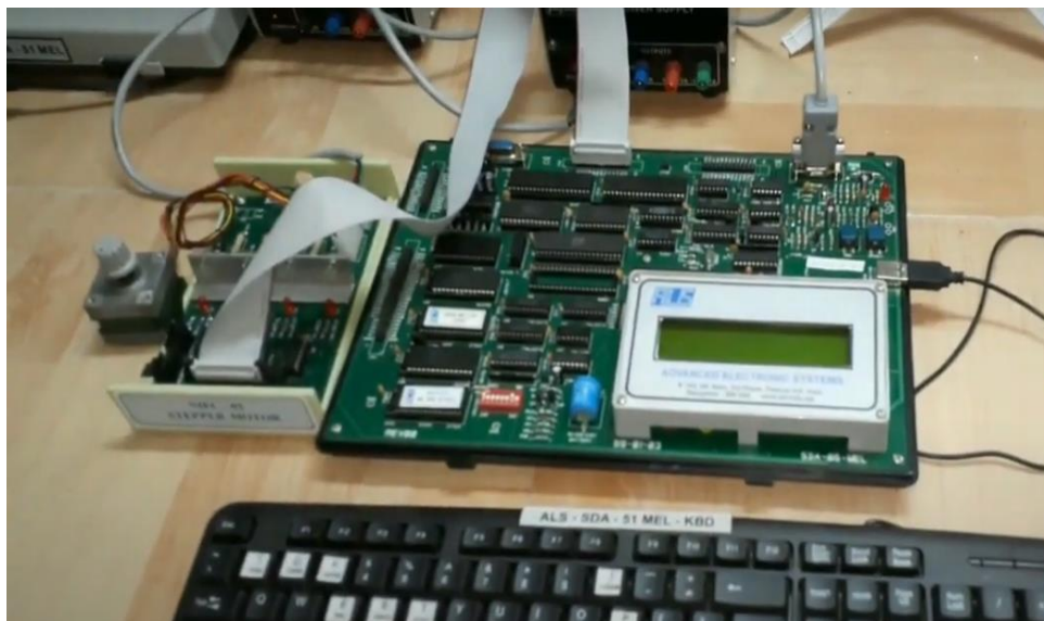
Figure 7: Interfacing of stepper motor with 8086 microprocessor kit
